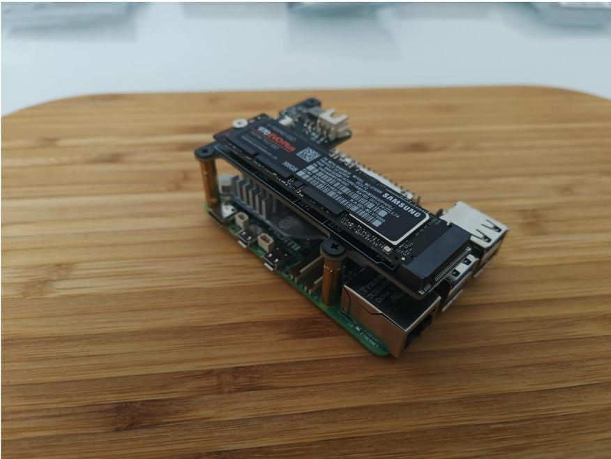
3. Then you need to install the Thermal Pad on top of the NVMe.
